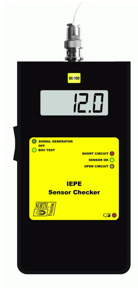
Figure 7: Good Bias Voltage Indication
