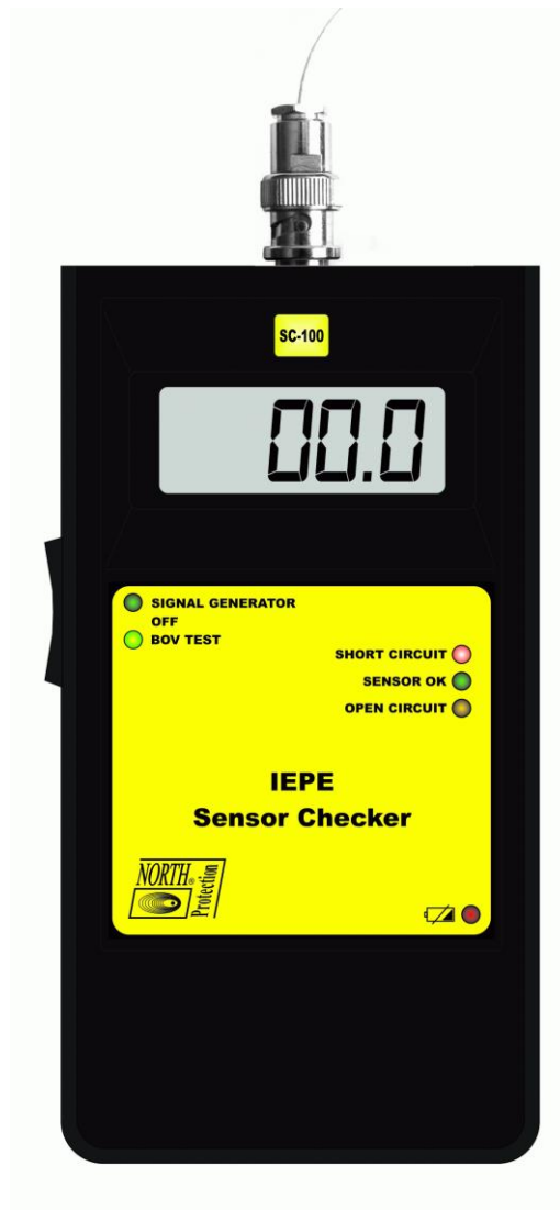
Figure 6: Short Circuit Indication
