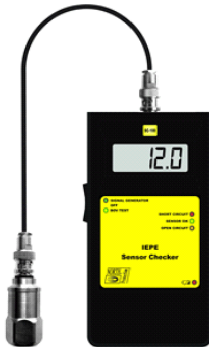
Figure 9: BOV TEST Mode, – IEPE (ICP®) Sensor Checking
