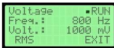
Figure 6. Sensor Simulator in Signal Generating Mode
