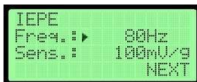
Figure 8. First step in IEPE sensor simulation
