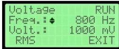
Figure 5. Change of Frequency in mV mode
