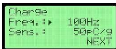
Figure 18. Selection of wanted frequency and sensitivity
