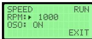
Figure 27. Choosing appropriate RPM and activating OSO ® screen
