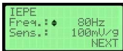
Figure 9. Screen for change of frequency
